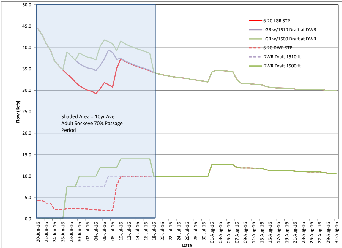
Figure 1. 6-20-16 STP flows at both Dworshak and Lower Granite as well as flows if the additional draft water from Dworshak (126 Kaf to 1510 feet and 244 kaf to 1500 feet) were used from 6/27/16 to 7/18/16 (shaded area in Figure representing the 10yr 70% passage date for adult sockeye passage at Lower Granite).
