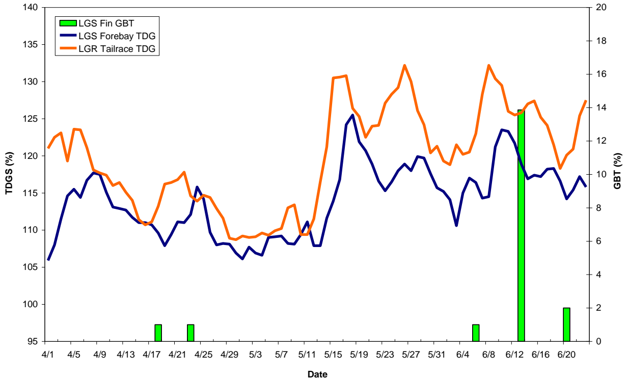
Figure 3. Percent of fish examined at Little Goose Dam showing signs of fin GBT with associated dissolved gas saturation levels in the Little Goose Dam forebay and the Lower Granite Dam tailrace.
