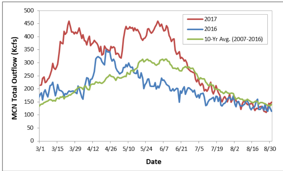
Figure J-2 Average daily flows at McNary Dam 2017, 2016 and the 10-year average
