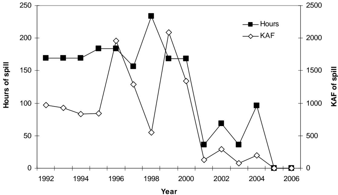
**Figure 1.** Hours of spill and KAF of spill at Bonneville Dam during the March release of Spring Creek NFH tule fall Chinook, 1992-2006.
